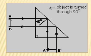
This action of prism is used in a periscope
