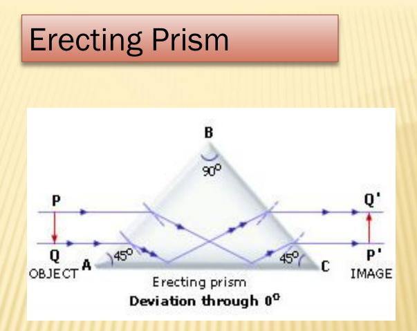
This action of prism is used in a slide projector
