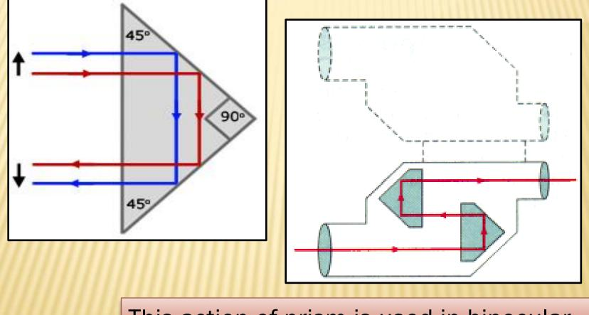
This action of prism is used in binocular
