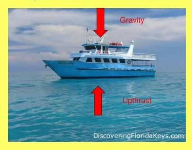
This boat has gravity pulling it down, and the upthrust of the water pushing up. Because the forces are balanced, the ship floats.
