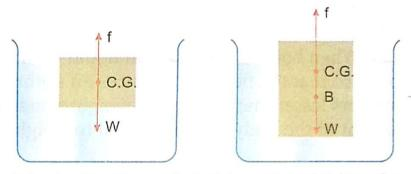
below the centre of the gravity *G* of the entire body. The weight of the body acts at C.G. (downwards) but the upthrust acts upwards at point *B* and both weight and upthrust are equal.
