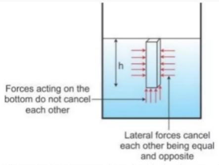
When a body is immersed in a liquid, the thrusts acting on the side walls of the body are neutralized as they are equal in magnitude and opposite in direction. However, the magnitudes of pressure on the upper and lower faces are not equal. The difference in pressure on the upper and lower faces cause a net upward force (= pressure x area) or upthrust on the body.
