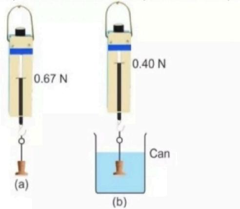
Take a solid body and suspend it by a thin thread from the hook of a spring balance as shown in the above figure (a). Note its weight. Above figure (a) shows the weight as 0.67 N.
